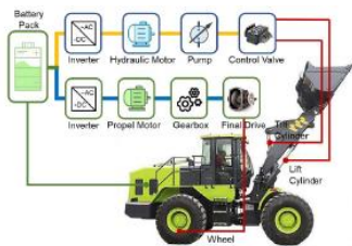
Figure 1: Powertrain of the electric wheel loader
